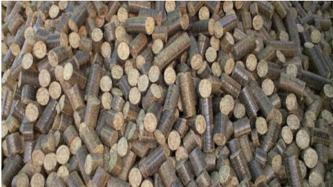
Groundnut Husk + Coffee Husk + Saw dust = Biomass Briquet
